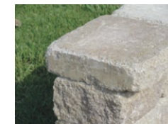
Parapet Cap 3 5/8" x 15 5/8" x 13" wt: 56 lbs. qty/pallet: 45
